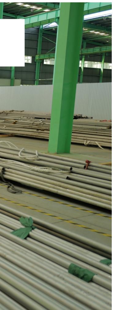
All machine automatic. First cold drawn from 65mm OD to 38mm. Then heat treatment.
