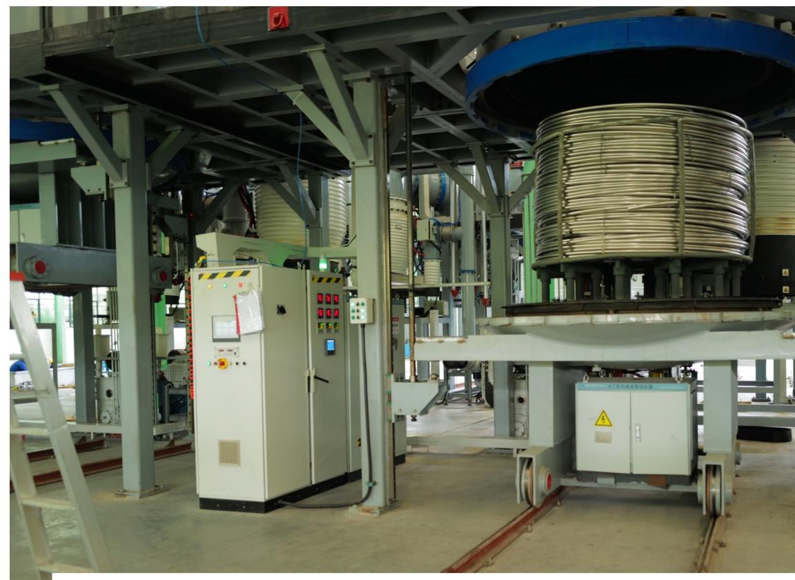
The dimension from 24mm down to 4.76mm accomplished by repeated cold pull, cleaning and heat treatment.
